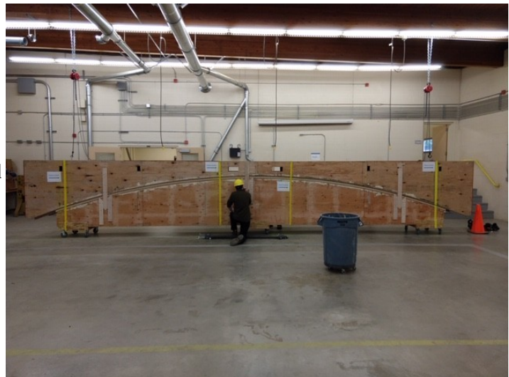
Form for building laminated siding planks: 2016
