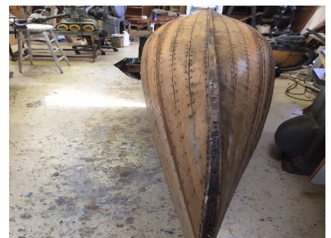
Even after 100 years, the cedar planking is tightly fitted.
