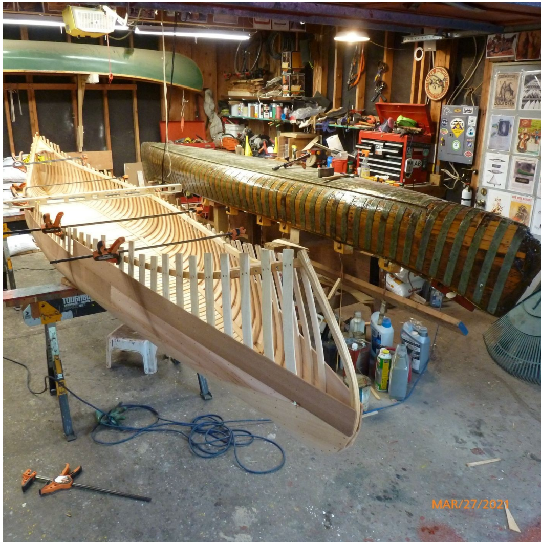
Martin Ferwerda is building a new 18' Thompson "Hiawatha" using the original Thompson factory form he restored. Ferwerda photo
