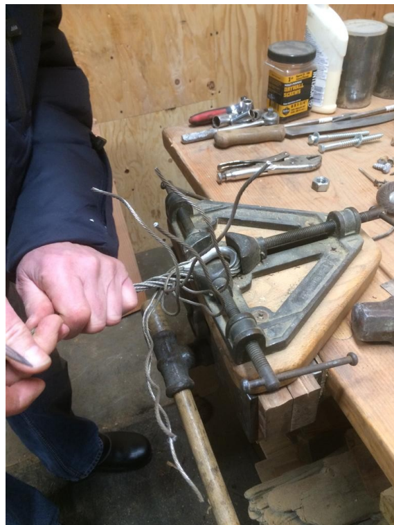
Eye splice for new rigging. M. Davidson photo
