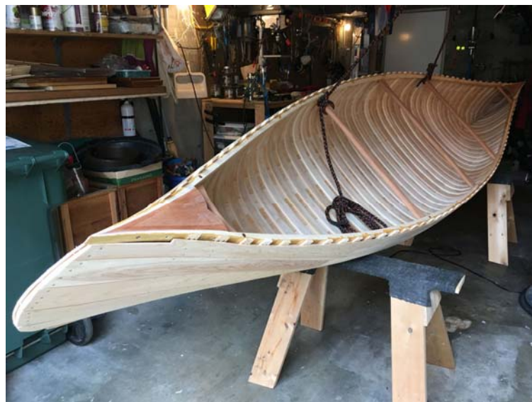
2,000 tacks, clinched – the canoe is ready for interior varnish.
