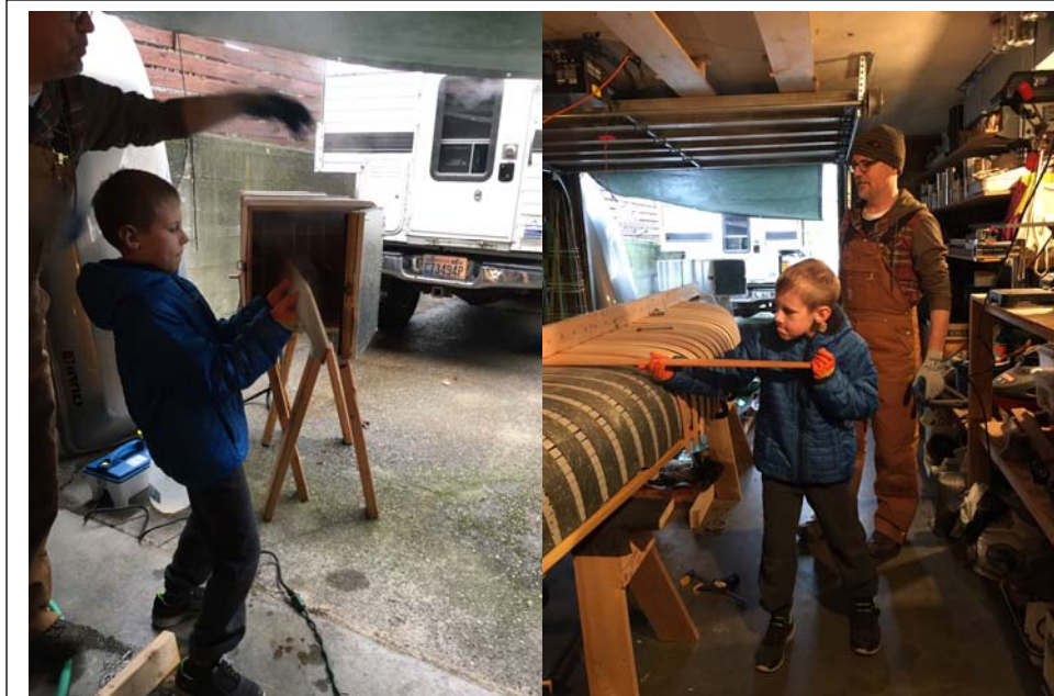
Matthew removes a rib from the steam box and then installs it.
