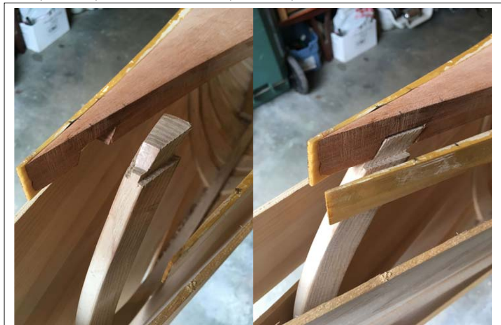
A mortise cut into the deck traps a tenon on the end of the stem.
