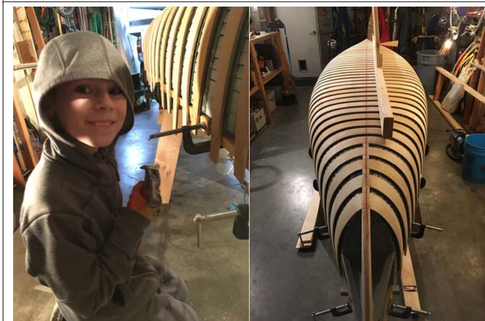
Matthew nailing ribs to the inwale. Forty-four ribs, bent on!
