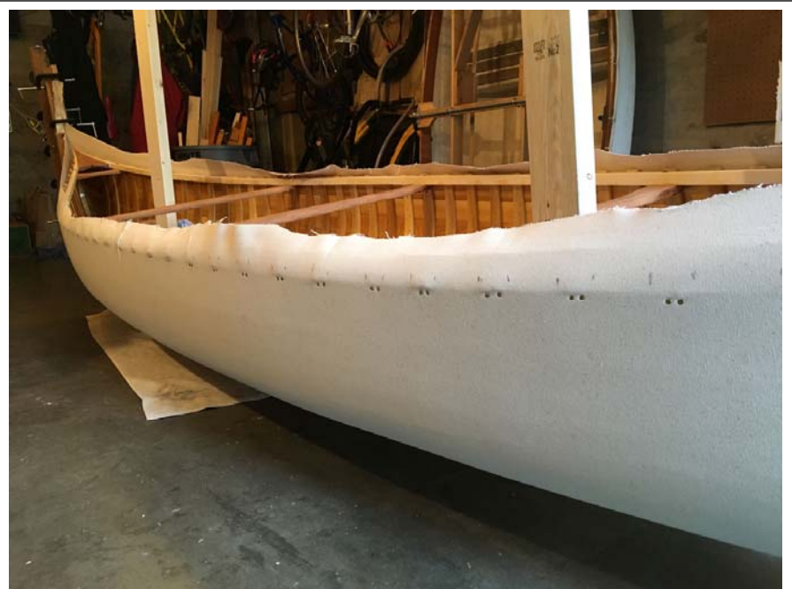
The canvas tacked onto the hull at the shearline.
