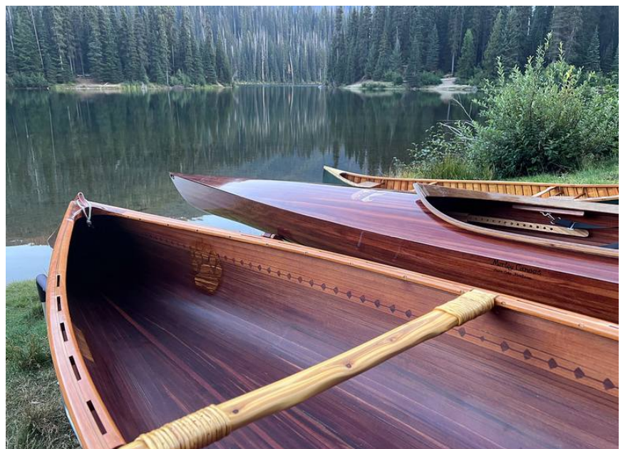
Morely Kootenai canoe showing grizzly track, sturgeon lateral markings, and spruce root lashings. Livdahl photo
