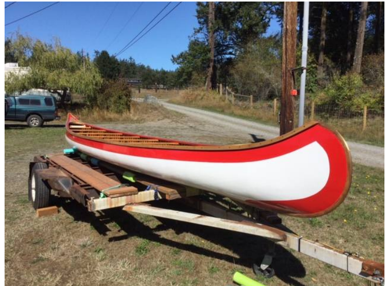
Completely refurbished with new fastenings, rib and planking repairs, new canvas and paint, the canoe is ready for more happy campers. Heikkila photo
