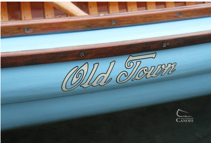
Mahogany outwales and rub rails on the sponsons contrast with the glossy new paint and decals. Mike Elliott photo
