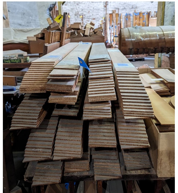
Shop contents in the warehouse: milled planking stock. Form for bending midsection of canoe's inner planks in the background. McElroy photo
