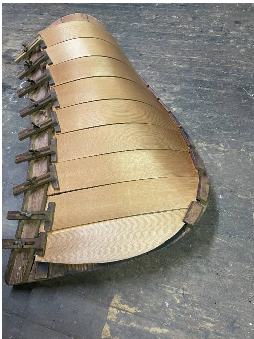
Each plank piece for the canoe ends has a distinct, individual curve. Phil Miller photo
