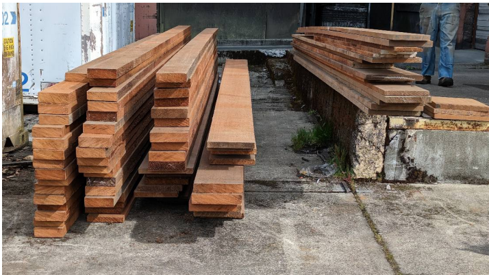
Clear red cedar boards await the arrival of the truck. McElroy photo
