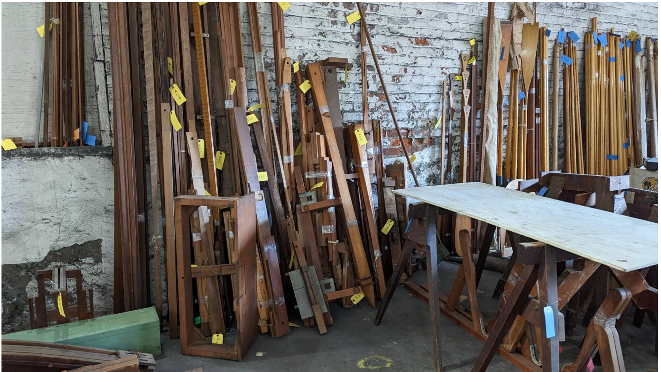
Shop contents in the warehouse: note paddle patterns, home made measuring sticks with hand lettering, trim stock, new oars and sailing rig spars. McElroy photo
